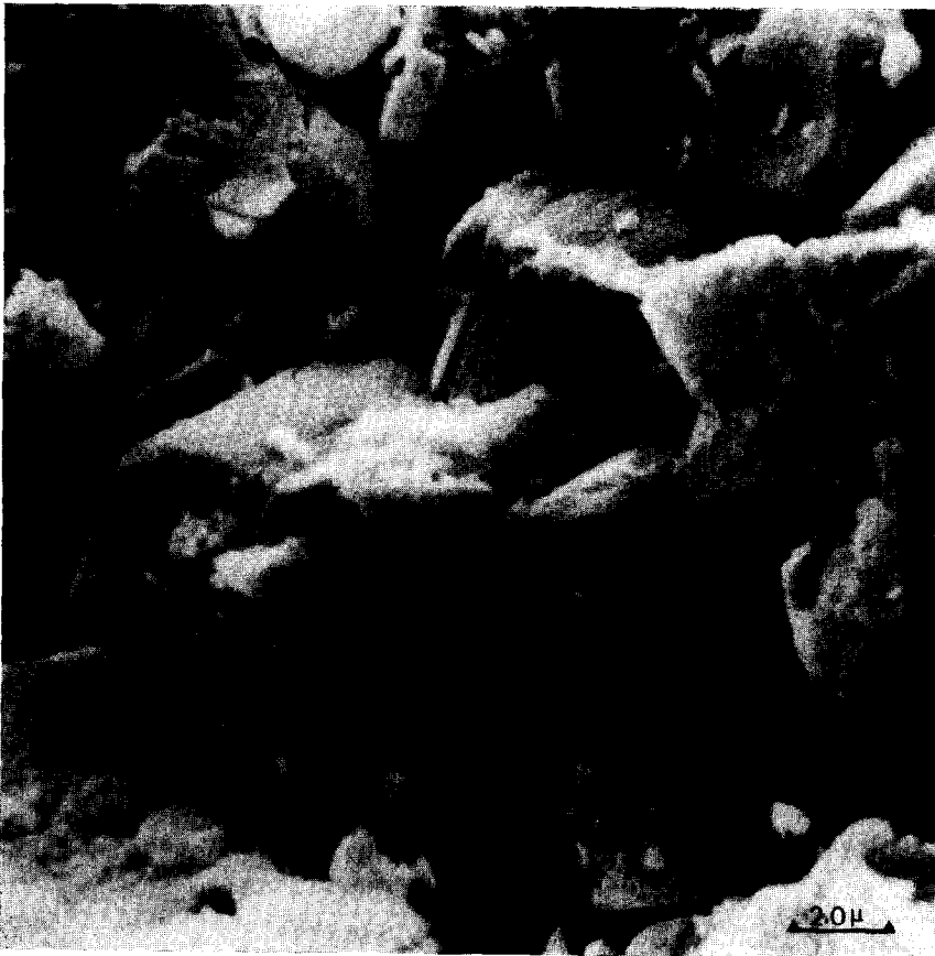
FIG. 4. Scanning electron micrograph of alumina pellet (low magnification; \times 5850 ).
